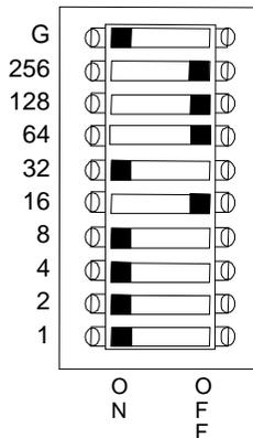
The DIP switch example above shows a station address of 208.
