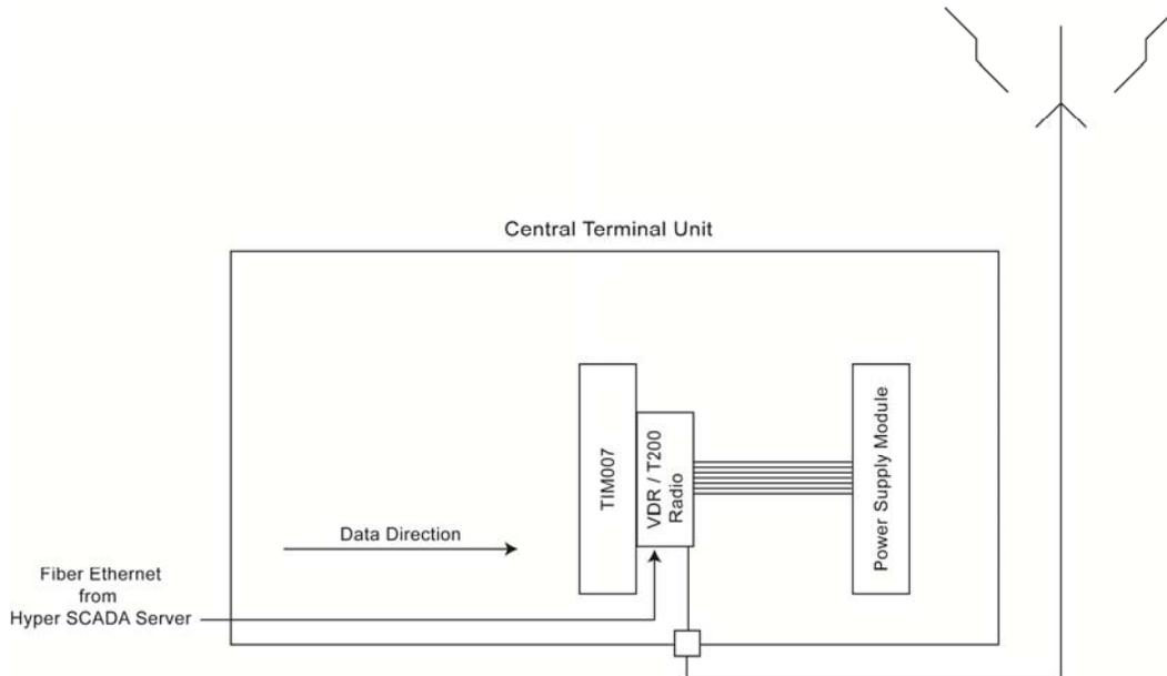
Figure 5-2, CTU with Voyager in High-speed Mode
