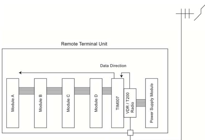
Figure 4-2, Typical TAC II Protocol RTU Configuration
